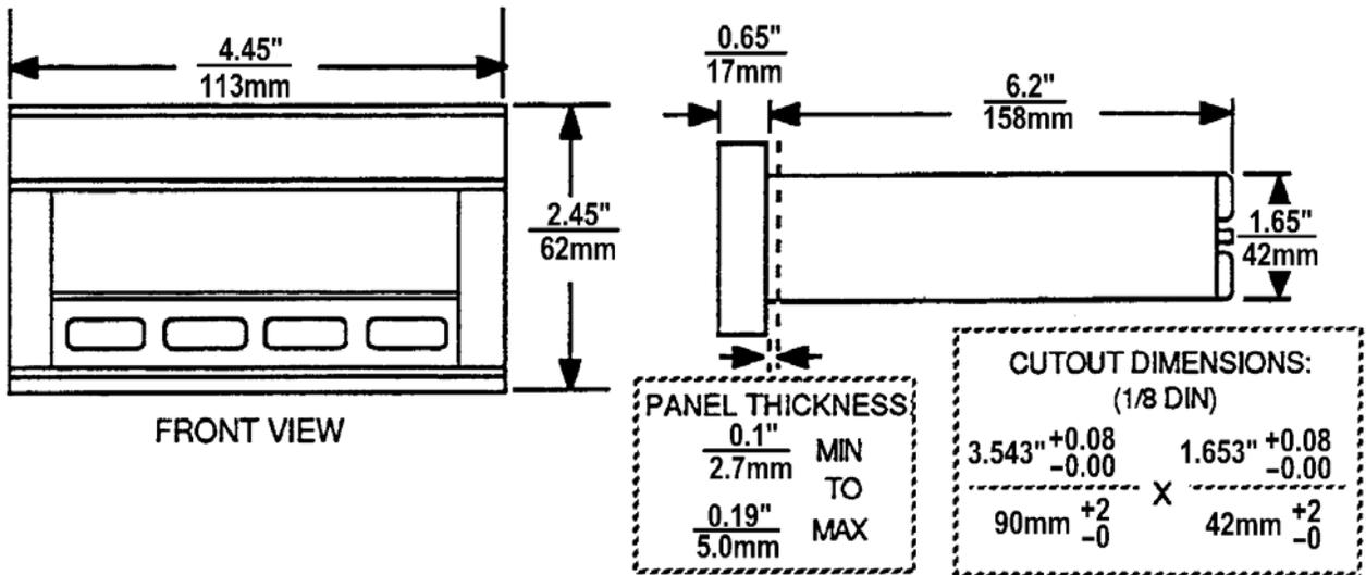
Figure 1.1 Mechanical Dimensions
