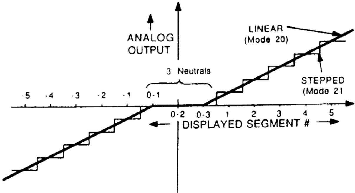
**Figure 2.5 Bi-polar Mode Analog Output**
